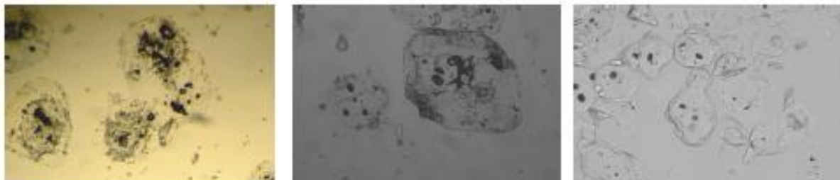
Figure 4: Images of energetic crystals from different batches, studied using optical microscopy with crystals submerged in index-matched fluid, to show internal structure more clearly. Less voids required higher shock pressures to cause reaction [16].
